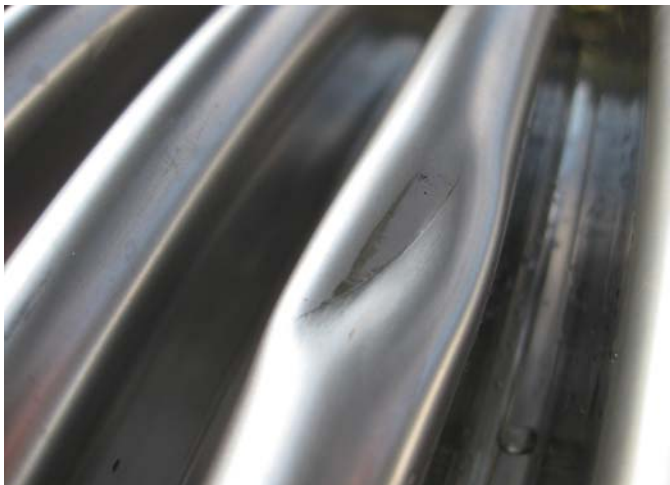
Shallow dent - Unsightly, yes. Time to replace? No.
