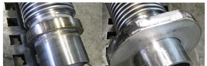
*Low profile shear pad (on left), floating ring added (on right)*
