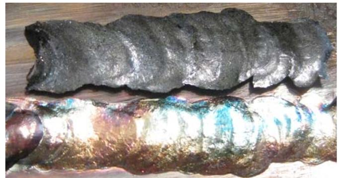
*Top side of repair weld using flux-core – note protective slag*
