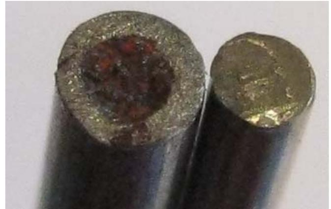
*3/32" Flux-core TIG wire vs. equivalent 1/16" TIG wire*
