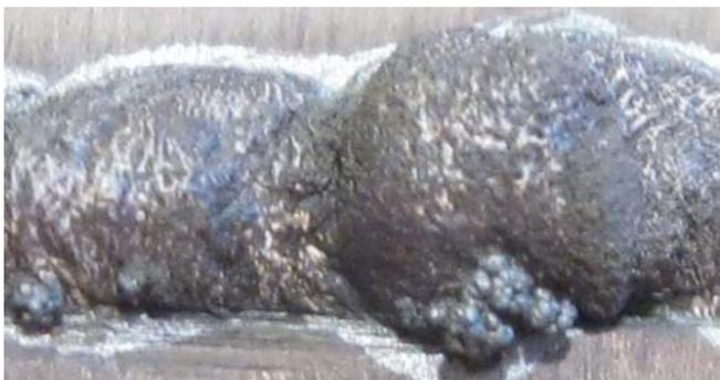
*Burn-through of weld with no shielding gas or flux – note 'sugaring'*
