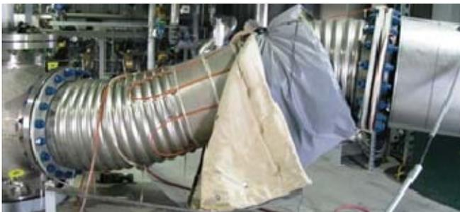
*Unsupported pressure thrust extends expansion joint metal bellows*
