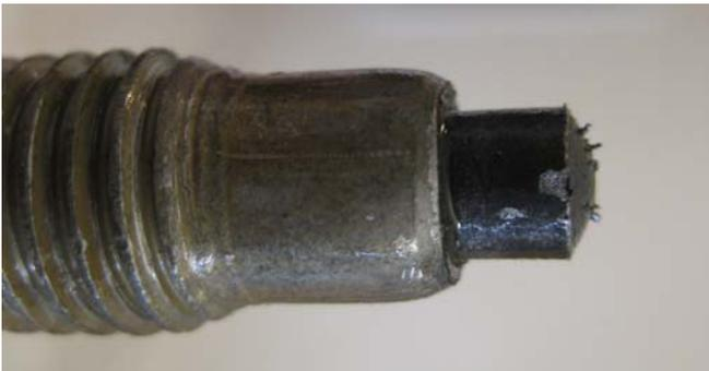
Magnetic oil drain plug with engine metal fragments from my 2005 GMC Truck - 124K miles (I dissolved oil from the plug with WD-40)
