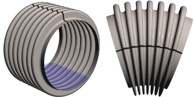
For expansion joint applications where the major movement is angular (hinged) or lateral (tied universal) a bellows long-seam that is aligned in the same plane as the neutral axis of movement will see little to no flexing – thus relegating the weld's only job to that of pressure containment.
