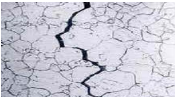
Intergranular crack - 'the crack goes around the grains'
