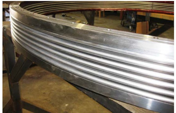
Stainless steel bellows quietly protected by a thin layer of chromium oxide
