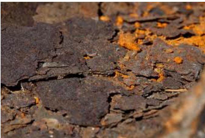
Iron oxide flakes away from carbon steel
